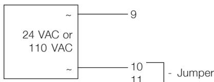
Two power supplies, one for sensor system and one for the solenoid valves:
