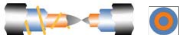
Fig 4. The unique tube-in-tube design. The orange areas show the product flow channel. These surfaces are electropolished.
